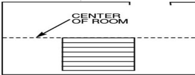
Avoid cutting in pieces less than half the plank width or tile size, if you find the cut in planks or tile will be less, the centre starting line should be moved to allow for minimum half the plank or width. This will “balance” the room and provide for a larger cut piece at the wall.
