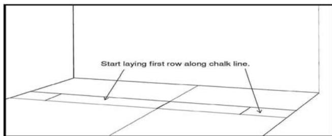
Start by placing a 2 metre straight edge on the floor along the centre line to keep the planks and tiles square.
