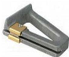
Overlap the second piece and recess scribe the seams using the Armstrong Flooring S-83 Recess scriber or by the trace cutting the join leaving a maximum gap of 0.5mm. Roll the cut edge into adhesive using hand roller. Roll seam and the entire floor using 45kg roller.
