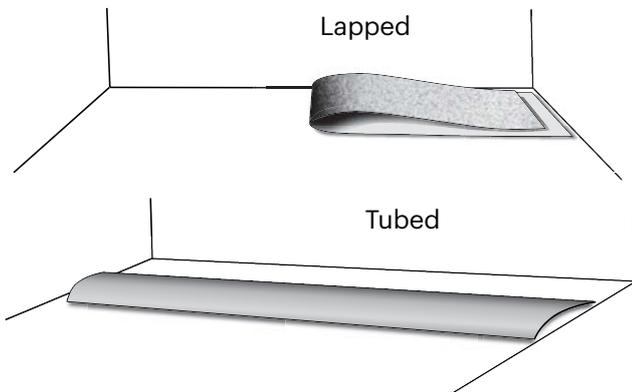
Spread the recommended Adhesive using the nominated trowel notch size. Allow adhesive to tack up, approximately 10/ 20 minutes depending on site and subfloor conditions. Lay vinyl flooring into the adhesive, using a push board, expelling any trapped air, then roll the vinyl with a 45kg roller in both directions.
