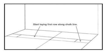
Start by placing a 2 metre straight edge on the floor along the centre line to keep the planks and tiles square.
