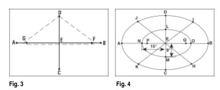
5. Mark R as the midpoint between EC and EH. Mark S, T, U, V, W, X and Y in the same way and draw lines from each of them. Draw lines CR, RH, HS, SB, BT, TI, IV, UD, DV, VJ, JW, WA, AX, XK, KY and YC to complete drawing the
