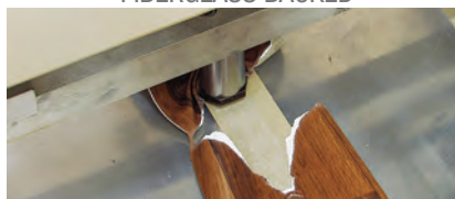
80 lbs. Results in Total Structural Failure
