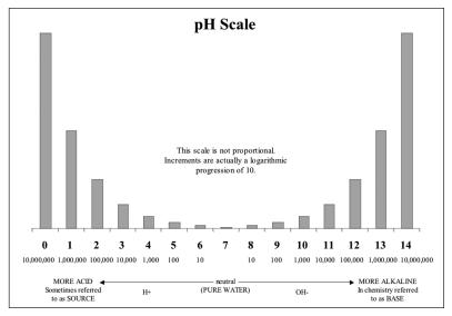
Rinsing and vacuuming with potable water is the best way to lower pH, but it cannot prevent the future deposit of salts on the surface of the slab. Do not use acid rinses to "neutralize" a high-pH concrete surface. The acid will deposit unwanted salts and can attack interior building finishes and be detrimental to the final installation.
